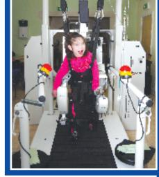
physical therapy is conducted with the aid of two or more therapists who manually move the patient's legs in a walking pattern. The strenuous nature and variability of the manual method can limit the frequency and duration of therapy. In the Lokomat, the robotic device does most of the heavy work, the pattern and pace are consistent throughout the session, and the exercise can be sustained over longer periods of time, making it more effective.
